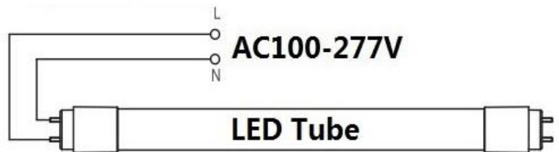
2. Two-End-Input : directly wire LED Tube in a fixture without ballast
