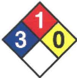
Note: The degree of hazard for flammability may be 3 in a confined space.
