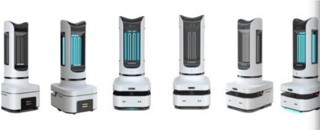
The **K-bot** is a general-purpose robot with wheel chassis and ultraviolet sterilization lamp. It is suitable for shopping malls, schools, families, office areas and other places where sterilization can be blocked.
