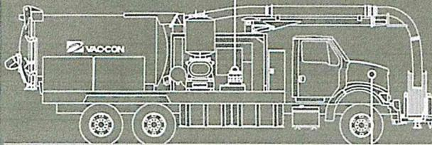
PD Blower powered by the Chassis Engine (275 horsepower)
