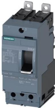
circuit breaker 3VA4 UL frame 125 breaking capacity class S 25kA @ 480 V 2-pole, line protection TM210, FTFM, In=20A overload protection Ir=20A fixed short-circuit protection li=15 x In clamp connection
