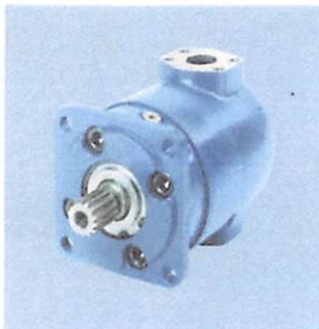
◀ MV015 – 2000 rpm 509 lb-ft (690 Nm) Offered in single, two-speed, double output shafts, wheel-bearing style, and retractable shafts along with splined, tapered, or straight keyed shafts. Through-hole and thrust bearing options also available. SAE C mount.
