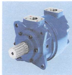
◀ MV015 – 2000 rpm 509 lb-ft (690 Nm) Offered in single, two-speed, double output shafts, wheel-bearing style, and retractable shafts along with splined, tapered, or straight keyed shafts. Through-hole and thrust bearing options also available. SAE C mount.
