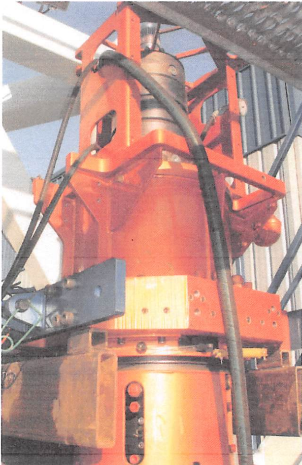
◀ Vane crossing vane motors power top drives for oil and gas exploration.
