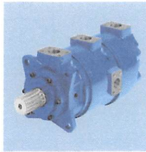
◀ MV037 – 1000 rpm 2007 lb-ft (2721 Nm) Offered in A [3000 psi (207 bar)] or D version [4500 psi (310 bar)]. Splined, tapered, straight keyed, and double output shafts are standard, along with through holes to 1 1/2". Optional thrust and radial load bearings with substantial capacity, tach pickups, double stacks (up to twice the torque), and brake mounts available. SAE D mount.
