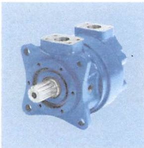
◀ MV037 – 1000 rpm 2007 lb-ft (2721 Nm) Offered in A [3000 psi (207 bar)] or D version [4500 psi (310 bar)]. Splined, tapered, straight keyed, and double output shafts are standard, along with through holes to 1 1/2". Optional thrust and radial load bearings with substantial capacity, tach pickups, double stacks (up to twice the torque), and brake mounts available. SAE D mount.
