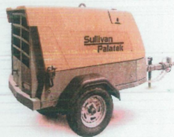
Internally the D185PKR is powered by a 48.8 hp Tier 4 Final Kohler engine and boasts a Sullivan-Palatek factory made 108 mm rotary screw air end at its core. The compressor also features side by side coolers for the compressor and engine, a large curbside toolbox for storage, a 10-hour full shift 30-gallon composite fuel tank with fuel level visibility, and a state-of-the-art curbside controller.
