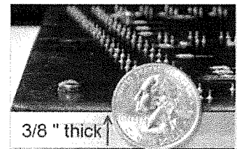
3/8" Bashplate protects LEDS
