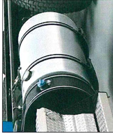
DEF tanks in three sizes complement your choice of fuel tank size and provide fill interval options appropriate for your application. Fuel tanks in 22" and 24.5" range in size from 56 to 150 gallons. Polished aluminum fuel tanks and polished stainless steel DEF tank covers are also available.
