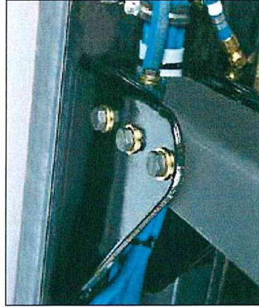
Heavy-duty crossmembers and 3-hole gussets strengthen the backbone of the T440 and T470, preparing it for the pounding your job dishes out. They can be replaced in less than 10 minutes with no special tools.
