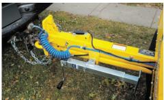
**TONGUE LENGTH.** A 60" (152.4 cm) tongue extension helps reduce the amount of repositioning needed on a jobsite.
