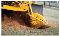
**AUTOSWEEP.** The patented AutoSweep® control system monitors engine speed and automatically adjusts cutter wheel sweep rate to maximize power to the cutter wheel while reducing engine stress.
