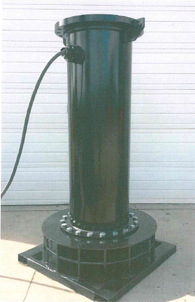
Example of Carrier Pipe for Axial Flow Pump (base to be modified)
