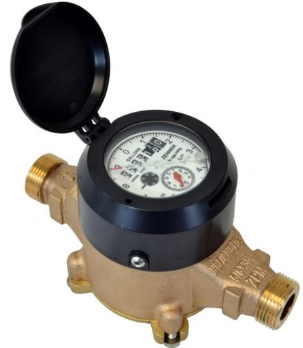
**INTRODUCTION:** ZENNER PPD Water Meters utilize a magnetically driven, positive displacement, oscillating piston design. It is designed to measure clean potable water where flow is in one direction only in residential, commercial and industrial settings.
