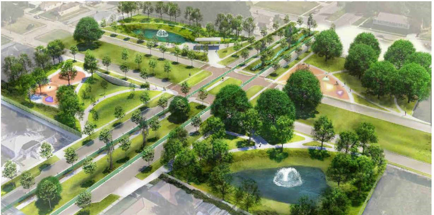
Blue and Green Corridors, New Orleans, LA. Four vacant lots in Gentilly are transformed into stormwater parks with site amenities and flexible storage for wet weather events.
