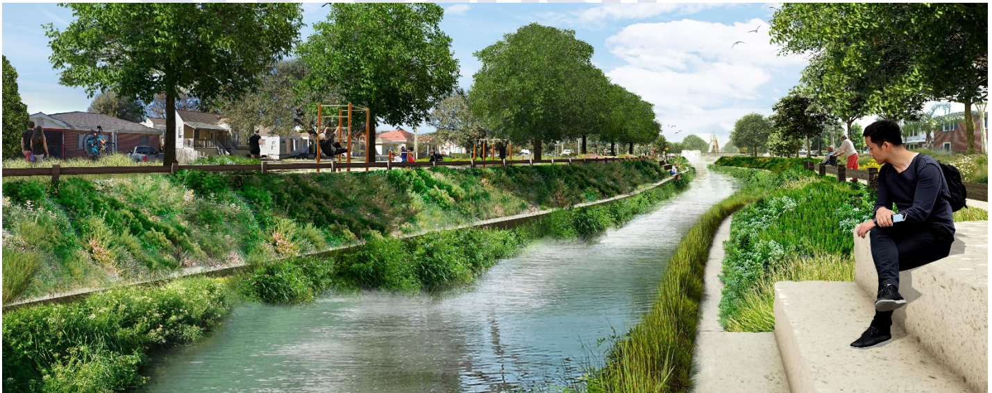
Blue and Green Corridors, New Orleans, LA. A raised neutral ground is transformed into a water feature that provides necessary flood storage and water quality benefits.
