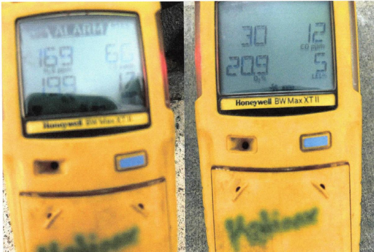
Hydrogen Sulfide = 169 ppm BEFORE
