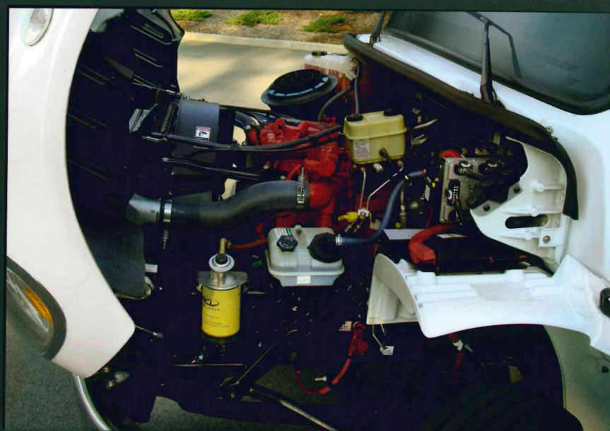
Tilt hood for easy engine access.
