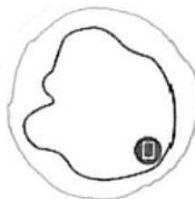
Figure 3. T750 5GHz Azimuth Antenna Patterns
