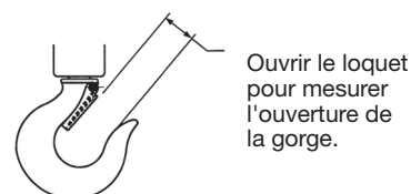
Figure 5 - Inspection du crochet
