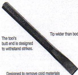
The tool's butt end is designed to withstand strikes.
