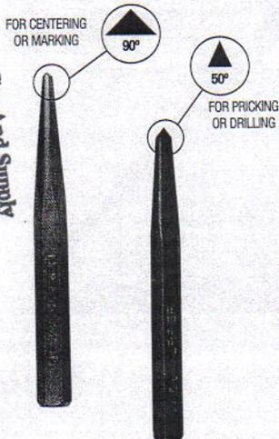
50° center punches are used to mark pieces in manufacturing or assembly. 90° prick punches are used to center the bore point and prevent tips from slipping off.
