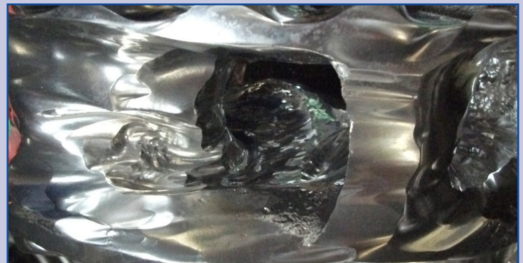
Impeller scoured by the sand mixture
