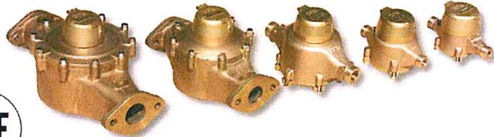
**INTRODUCTION:** ZENNER Positive Displacement Water Meters utilize a magnetically driven, positive displacement, oscillating piston design. It is designed to measure clean potable water where flow is in one direction only in residential, commercial and industrial settings.
