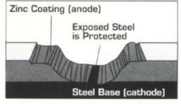
When Zinc is scratched the coating slowly sacrifices itself by galvanic action to protect the raw steel substrate.
