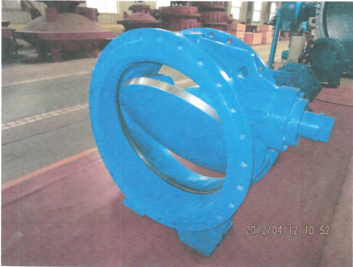
Tilting disc check valve
