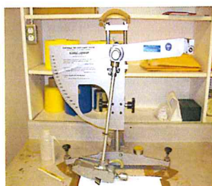
Skid-Resistance Tester
