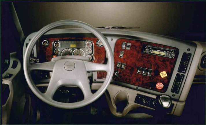
Advanced heating and cooling system features 14 vents, including one in each door, for uniform air distribution throughout the cab. Optional wing dash shown.
