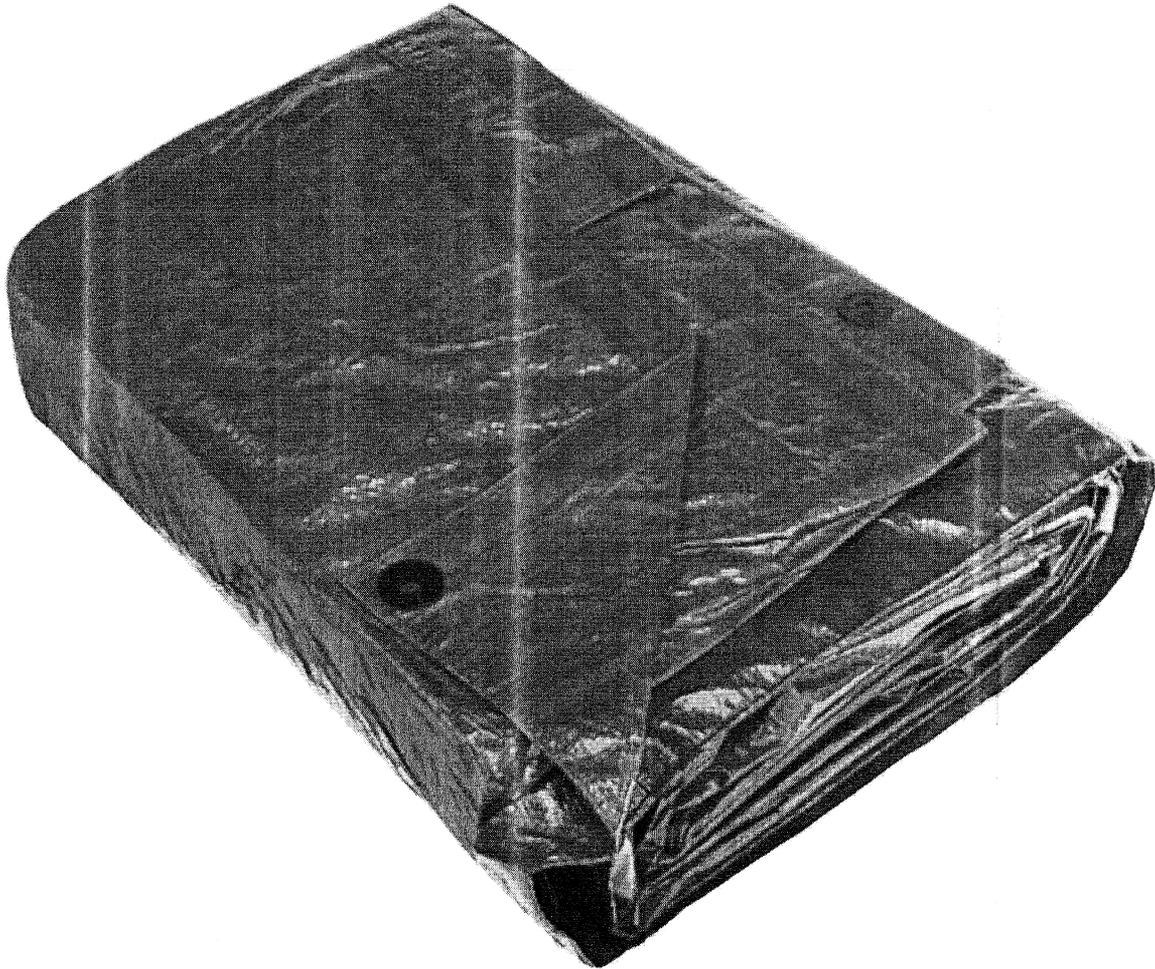
Grommets every three feet • Heat sealed seams • Reinforced hem
