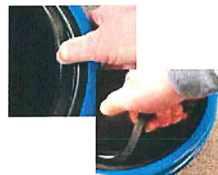
Use your thumb or other device to remove inner gasket layer.
