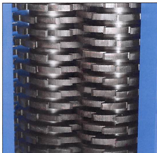
Twin shaft cutting chamber.
