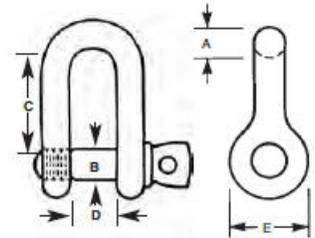
Screw Pin Chain Shackles meet the requirements of Federal Specification RR-C-271D Type IVB, Grade A, Class 2.
