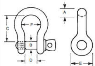
Screw Pin Anchor Shackles meet the requirements of Federal Specification RR-C-271D, Type IV A, Grade A, Class 2.
