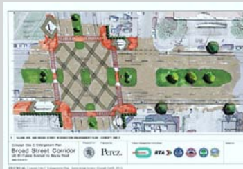
Proposed Broad Street Enhancements at Tulane Ave. showing decorative paving and rainwater irrigated tree well bulb outs in parking lane – New Orleans, LA
