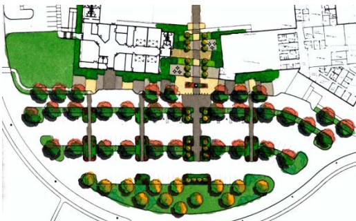
Plan of proposed enhancements including a parking lot containing bio-swales, native plantings, and a detention basin area to slow, reduce and clean storm water.
