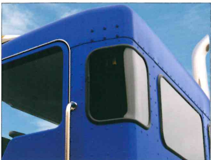
Cab corner windows greatly enhance visibility in tight places.
