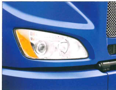
An advanced forward lighting system provides up to 30% more down-road coverage than conventional sealed beam designs. Choose the standard halogen or optional HID Xenon lamps.
