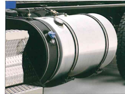
DEF tanks in three sizes complement your choice of fuel tank size and provide fill interval options appropriate for your application. Fuel tanks in 22" and 24.5" range in size from 56 to 150 gallon, to offer clear back of cab configurations.
