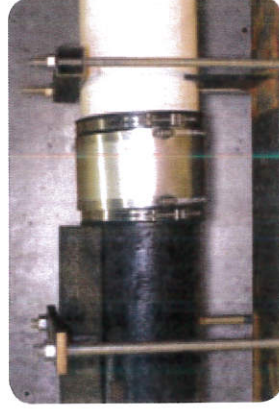
Shear Resistance Test using a Fernco 5000 Series Repair Coupling per ASTM C 1173 (applied load 50 pounds per nominal inch of pipe diameter)
