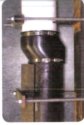
Shear Resistance Test using an unshielded sewer coupling per ASTM C 1173 (applied load 50 pounds per nominal inch of pipe diameter)
