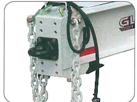
3" Pintle eye, with 4 adjustable height positions, with 2 heavy duty safety chains and grab hooks.
