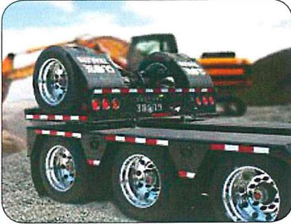
Globe Trailers flip axle design. It allows for less down time when operating the flip axle and it can be easily detached when required.
