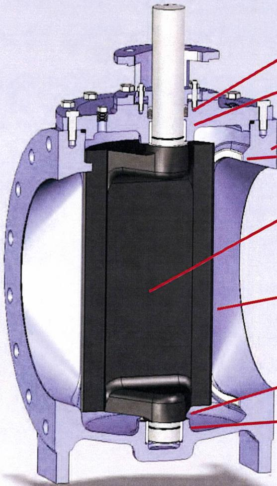
**Adjustable Packing**—Allows for maintenance and replacement of the packing without the removal of the actuator from the valve.
