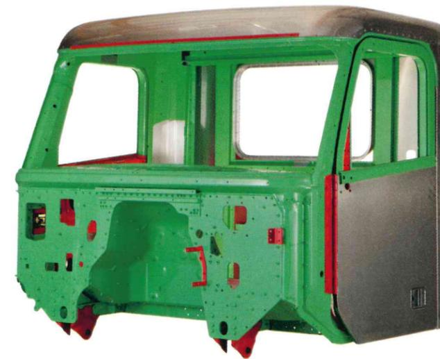
■ Aluminum Structural Reinforcements
