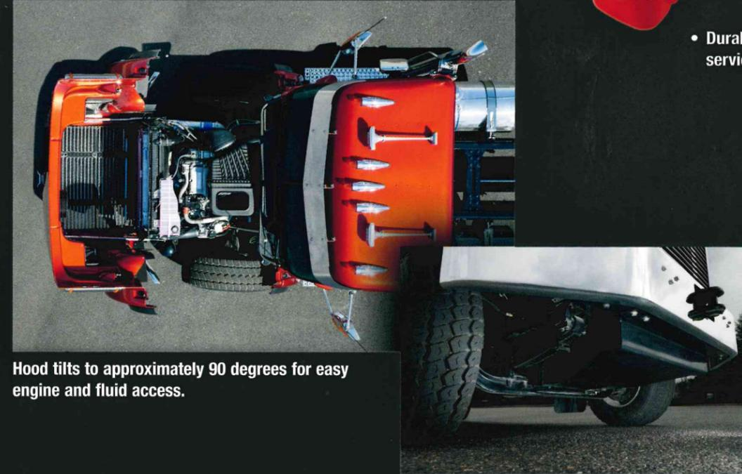
Hood tilts to approximately 90 degrees for easy engine and fluid access.
