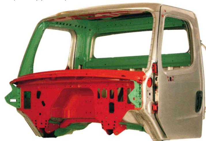
■ Aluminum Structural Reinforcements
