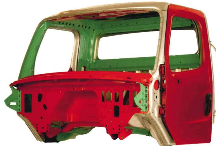
■ Aluminum Structural Reinforcements
