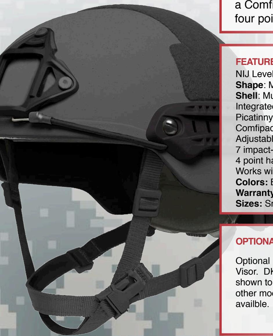
The Badger MICH/ACH III-A Ballistic Helmet is designed according to the latest US Military requirements utilizing the most advanced ballistic protection against gun ammunition. The shell is composed of multi-layered composite and comes with a harness assembly that consists of a Comfipad suspension system and a four point harness with leather chinstrap.
