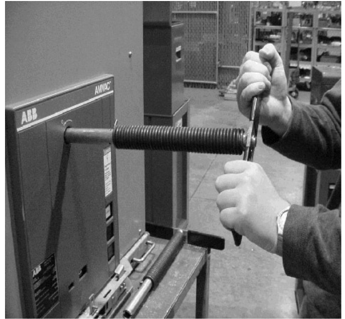
Figure 4: Manual Opening Handle Inserted
