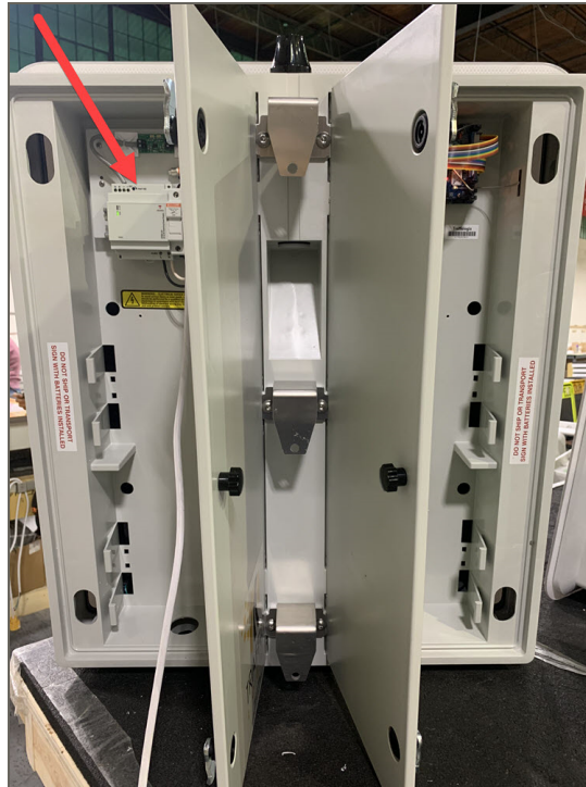
Figure 4: AC power supply terminal block location
