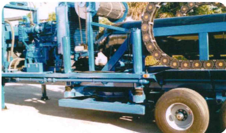
The turntable mechanism in traveling position.
