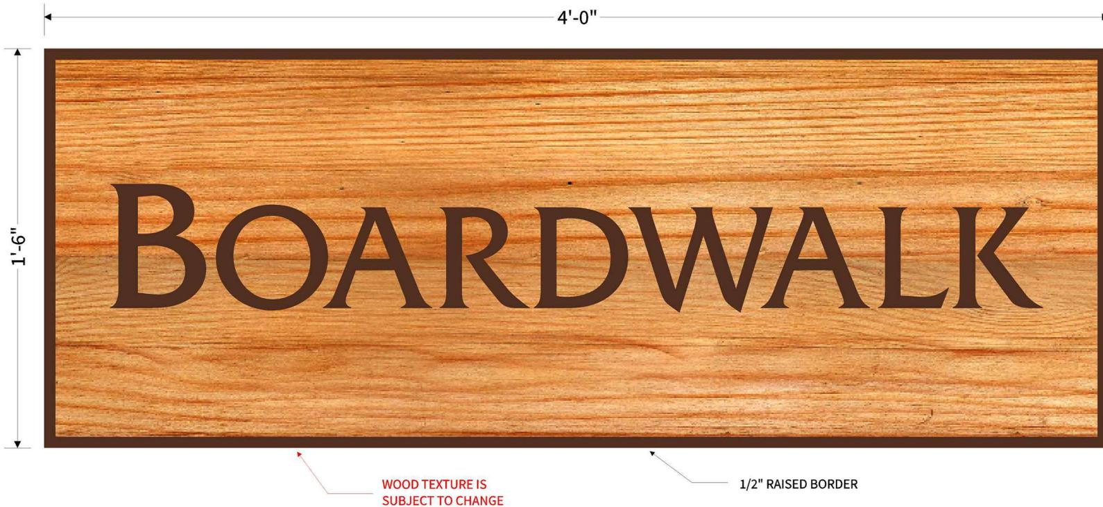
Manufacture & Install (2) thick custom made single sided carved HDU sign panel, raised text and border, faux wood grain painted background and wall mounted.
