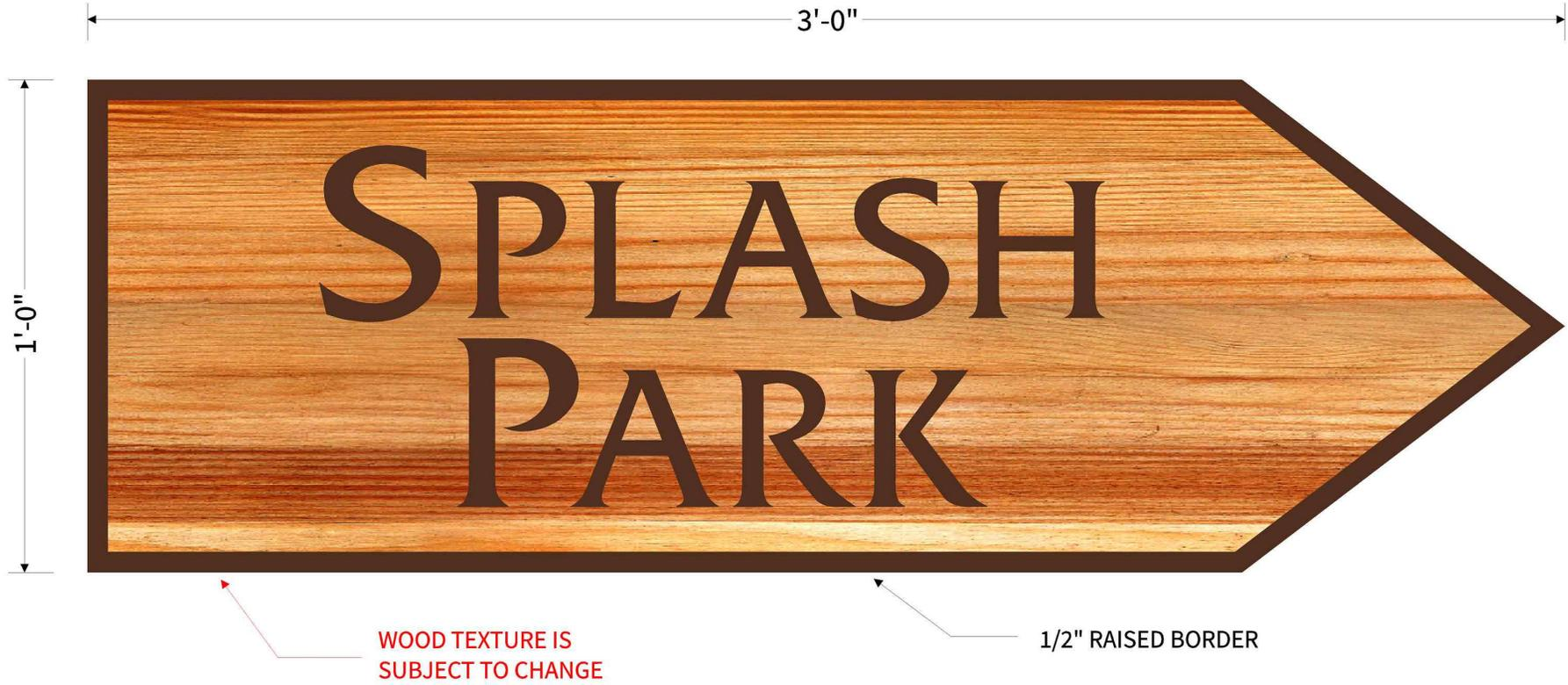
Manufacture & Install (1) thick custom made single sided carved HDU sign panel, raised text and border, faux wood grain painted background and wall mounted.
