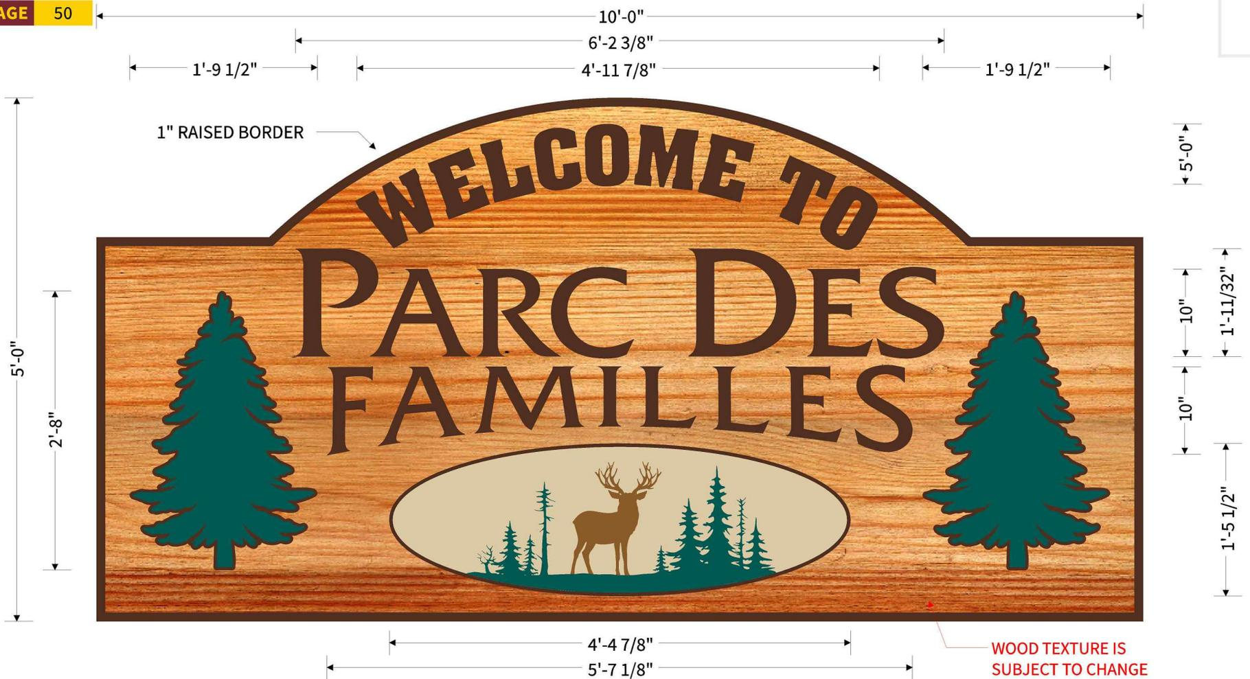
Manufacture & Install (1) thick custom made single sided carved HDU sign panel, routed down background in a wood grain texture finished, faux wood grain painted background and wall mounted.
