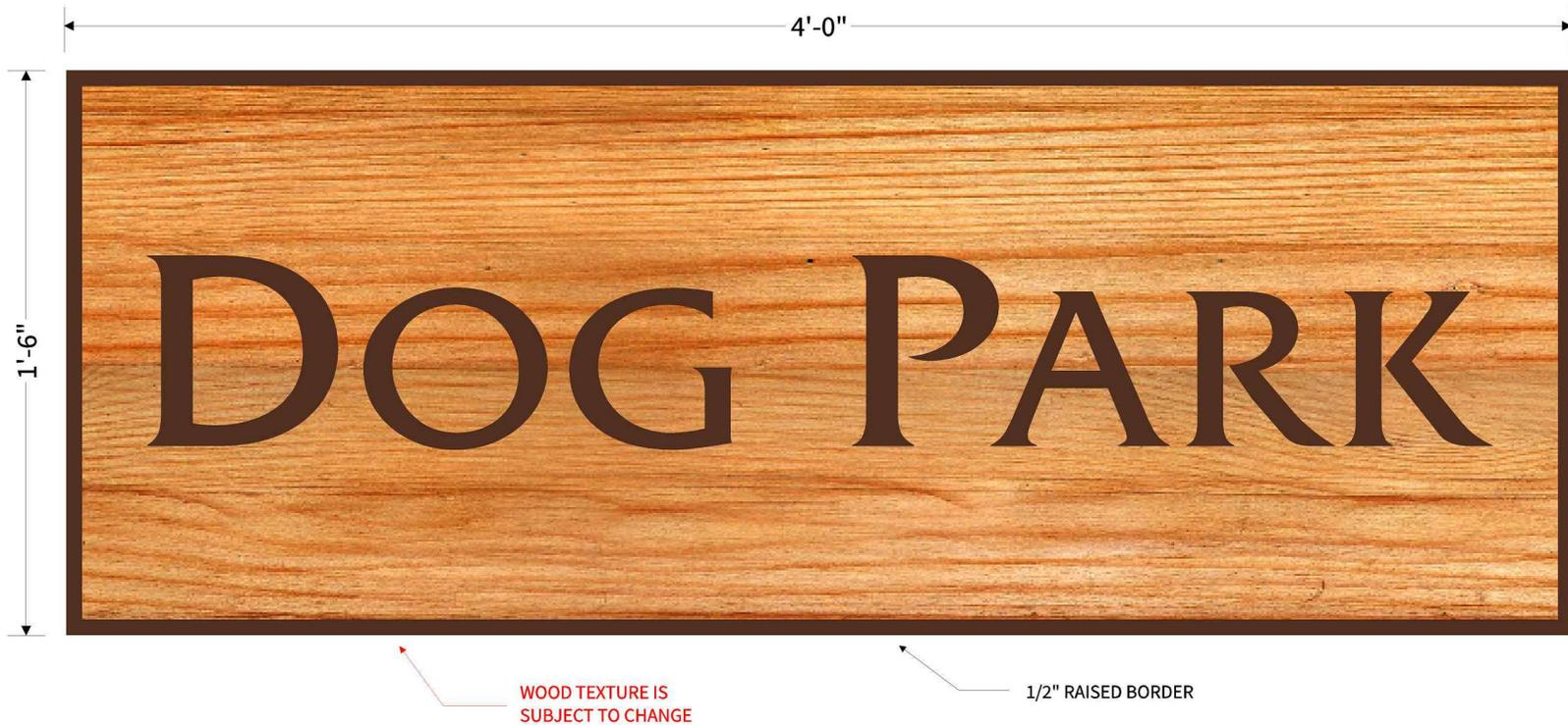
Manufacture & Install (1) thick custom made single sided carved HDU sign panel, raised text and border, faux wood grain painted background and wall mounted.
